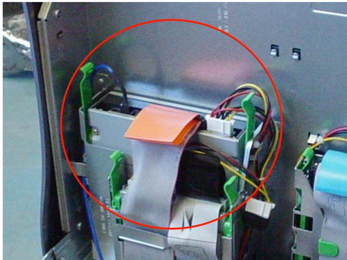
4. Remove the three connections to the CD-ROM Drive. Take care while removing them to hold them either by the connector itself or the orange pull tab attached to the cable.
