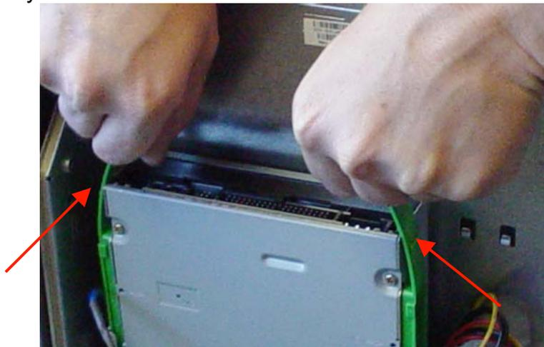
6. Insert the CDRW into the unit by holding it by the green handles and sliding it down the guides. The bay is keyed in the Server so that the unit will only fit in 1 way.
