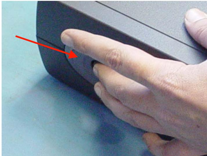
3. With the buttons pressed Lift the server open and locate the CD-Rom drive
