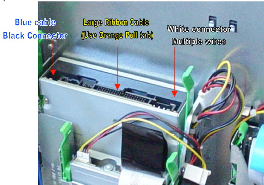
5. Remove CD-ROM by grasping the 2 green handles and lifting the unit out of the bay.
